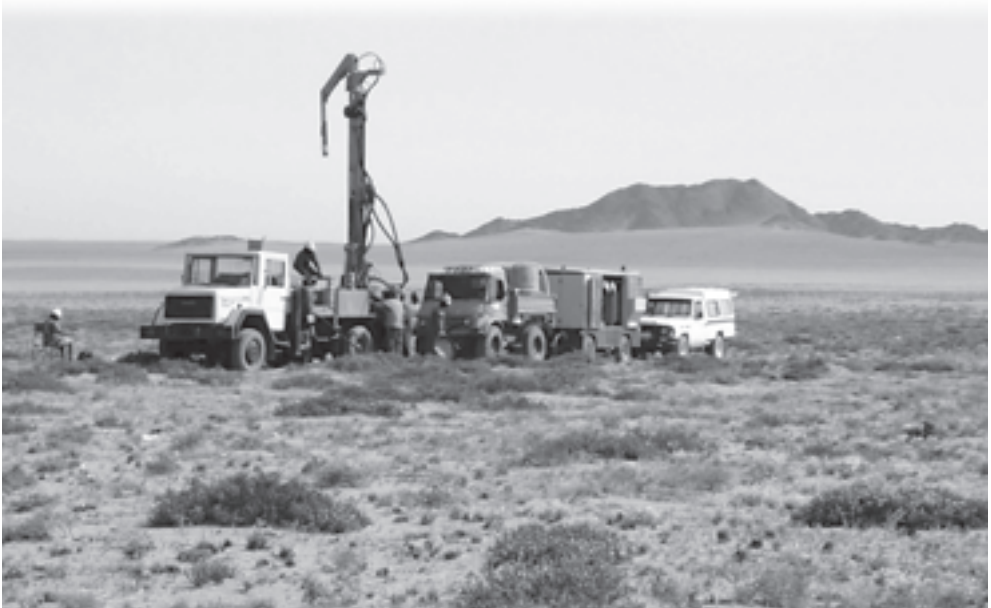
Rotary air blast rig in the Sperrgebiet of Namibia, showing how low impact activities can be managed in sensitive areas. Photo: Anglo American plc.
