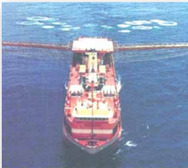
Survey vessel with airguns towed behind (Courtesy of UKOOA)
