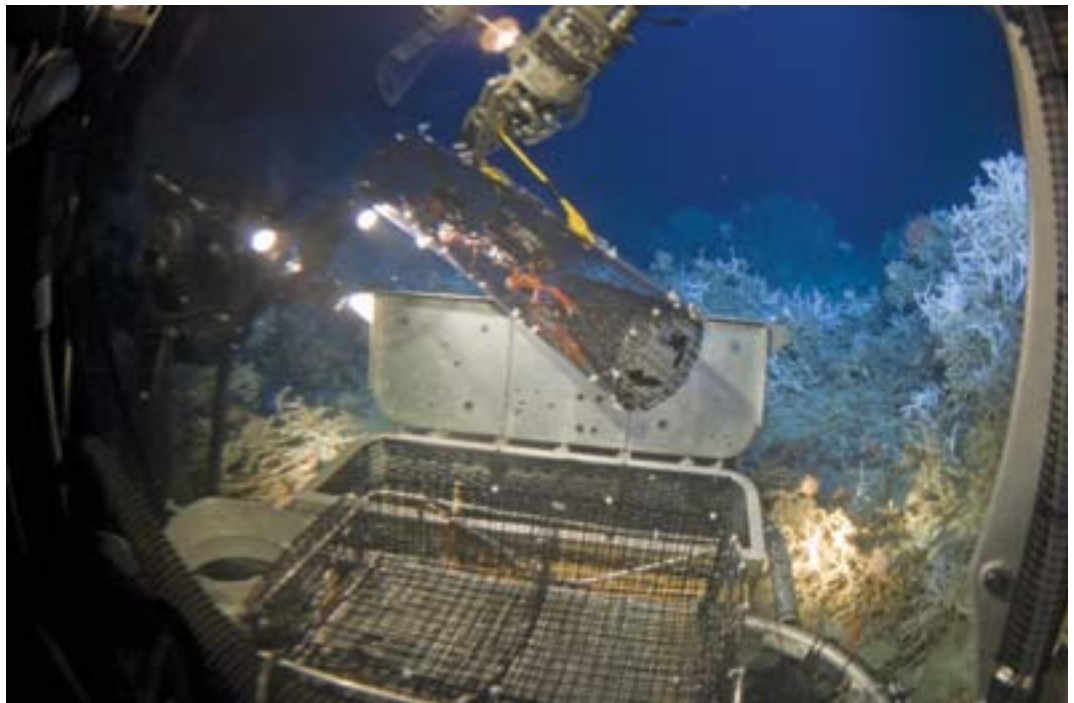
The submersible's manipulator arm collecting a crab trap containing five deep sea galatheid crabs. Photo Credit: Dr. Steve Ross, UNC-W. NOAA Office of Ocean Exploration.
